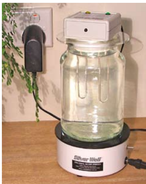
Generator, Stirrer Base, and Transformer.
